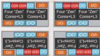
4 x 8-core Chiplet, 213mm 2 per chiplet 852mm 2 total area (+9.7%) 0.59x Cost
