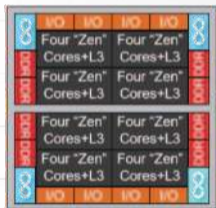
Monolithic 32-core Chip 777mm 2 total area 1.0x Cost
